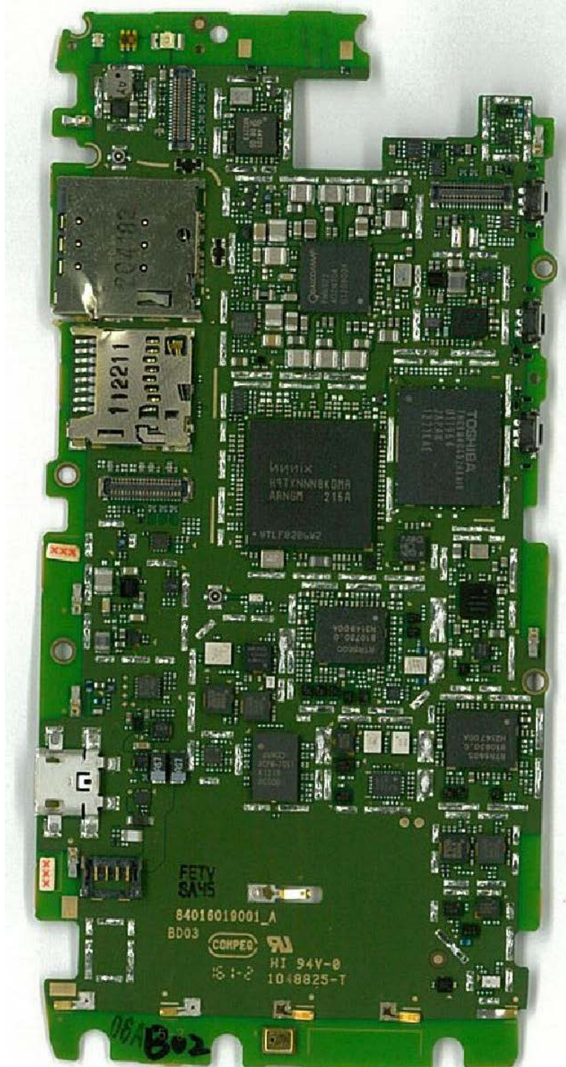
Photograph 9-2: Front side view of the device's PC Board, Shields Removed.
