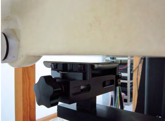
Fig.7 EUT front to flat phantom
