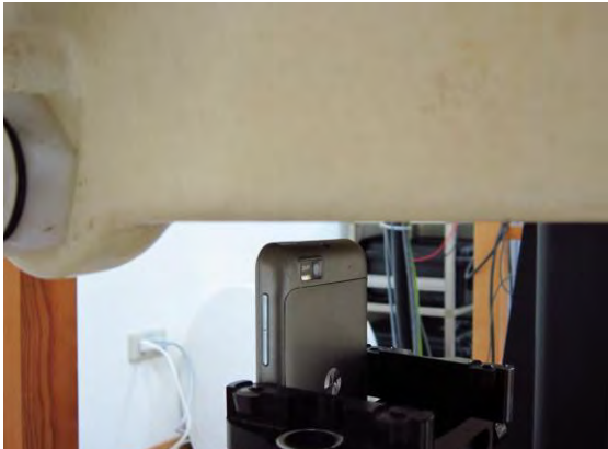
Fig.10 EUT Top to flat phantom
