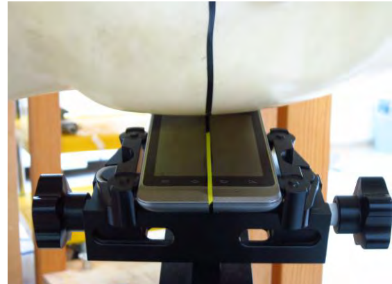
Fig.6 Left Head Section / Ear-Tilt Position(15°)
