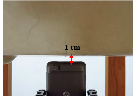
Fig.10 EUT Top to flat phantom
