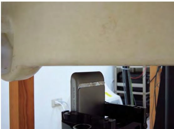
Fig.11 EUT Bottom to flat phantom
