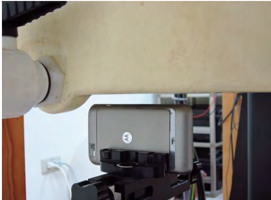
Fig.13 EUT Left to flat phantom
