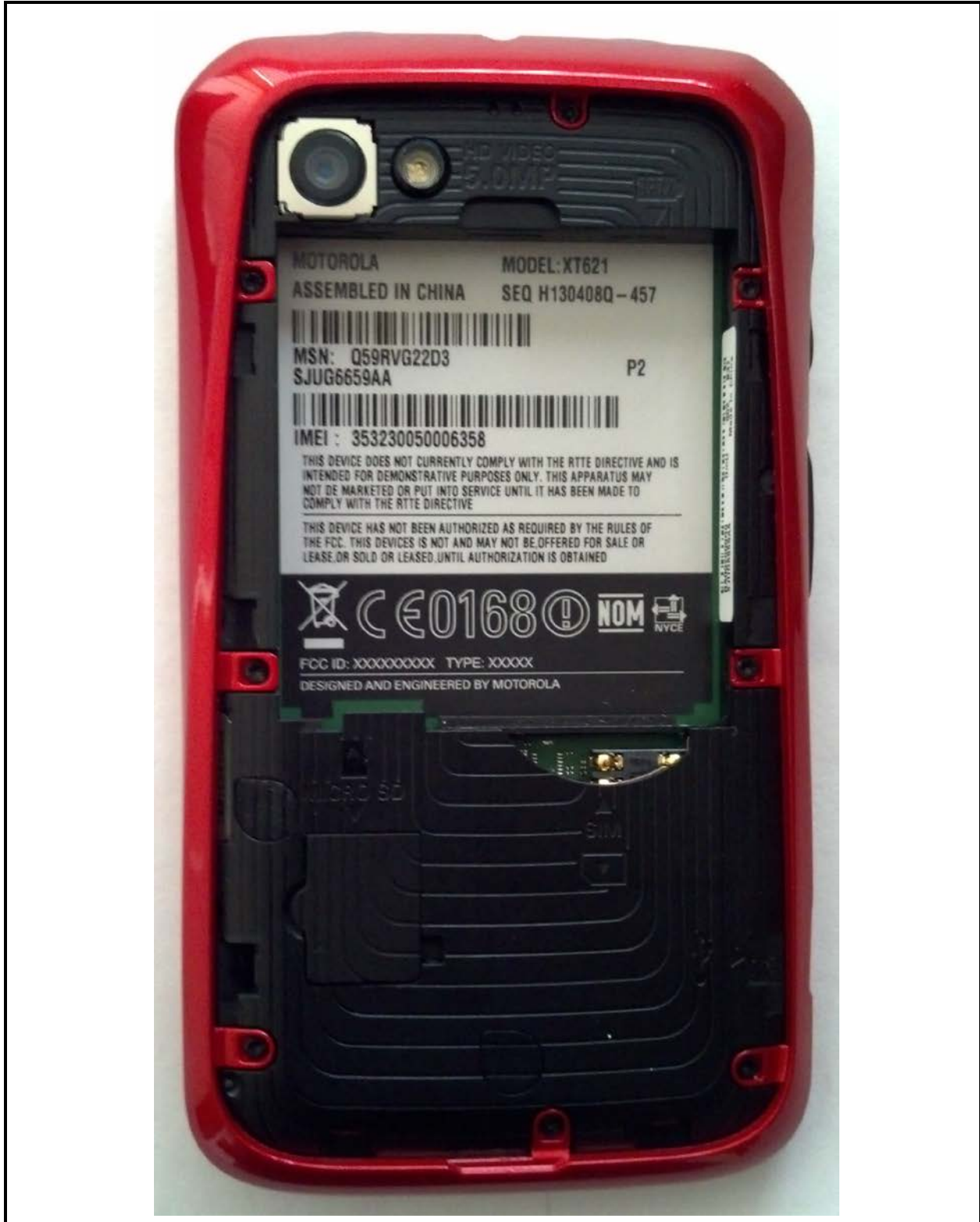
Figure 3-7. Detail of Regulatory Markings
