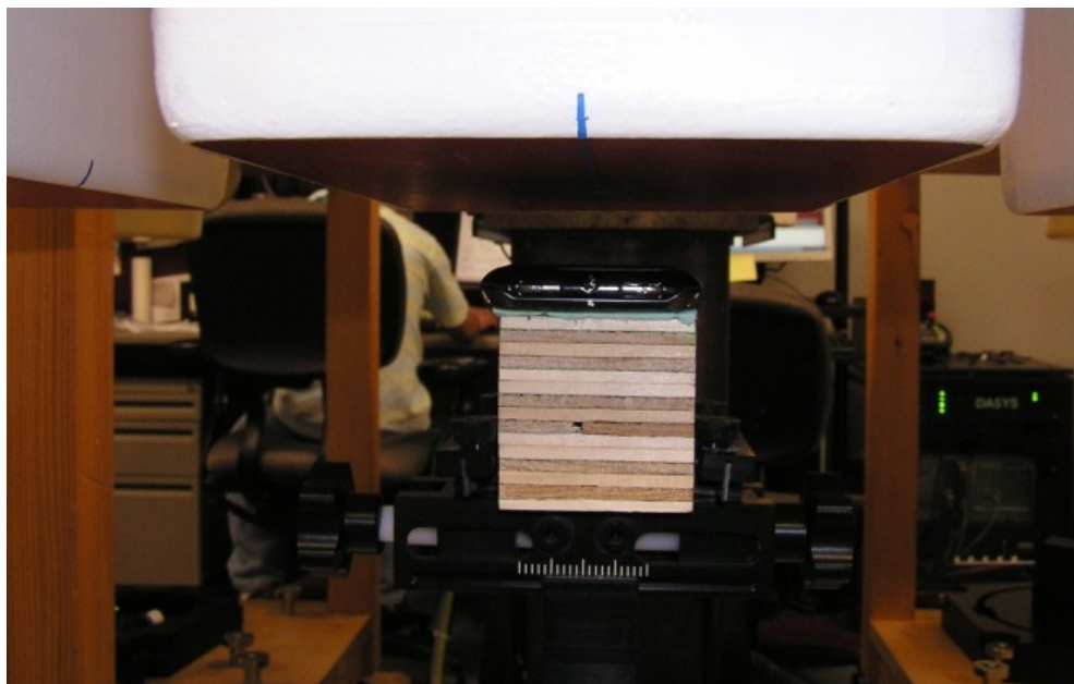
Figure 7: Mobile Hotspot Position, Back of Phone facing Phantom (10 mm separation)
