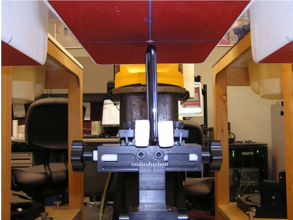
Figure 9: Mobile Hotspot Position, Short Edge (Top/Bottom) of Phone facing Phantom (10 mm separation)
