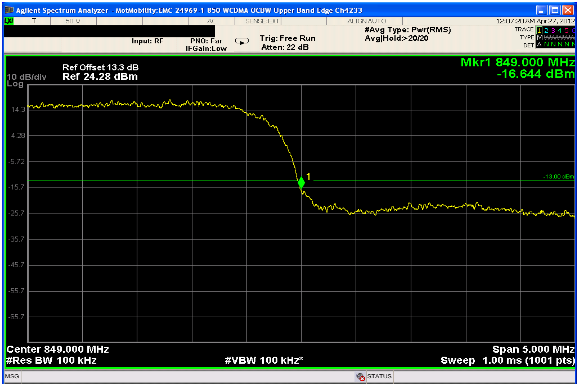
WCDMA 850 – Upper Band Edge – Channel 4233 (846.6 MHz)
