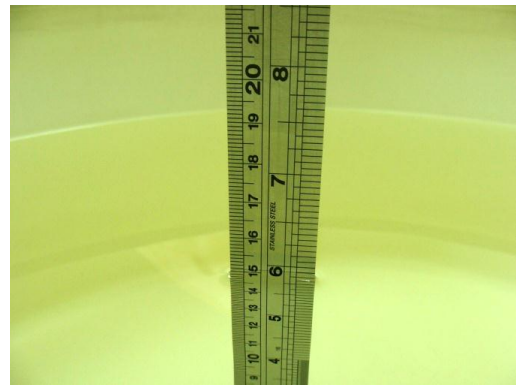
Fig 6.2 Photo of Liquid Height for Body SAR
