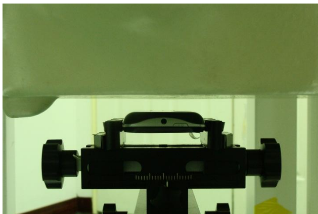
Rear Face of the DUT with Phantom 1 cm Gap (DUT without Earphone)
