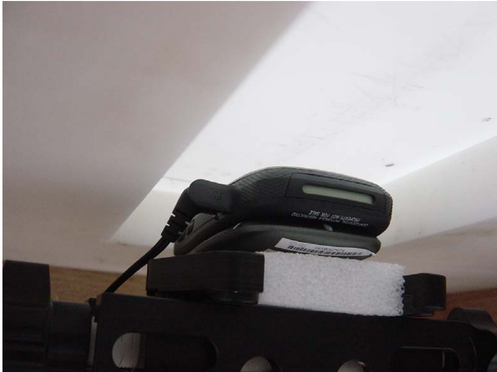
Figure 7: Phone Against the Flat Phantom
