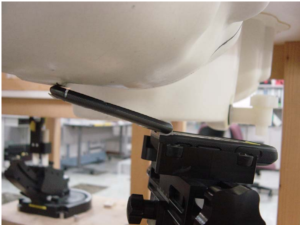
Figure 6: Phone Against the Head Phantom (15° Tilt)
