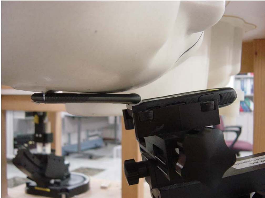
Figure 5: Phone Against the Head Phantom (Cheek Touch)
