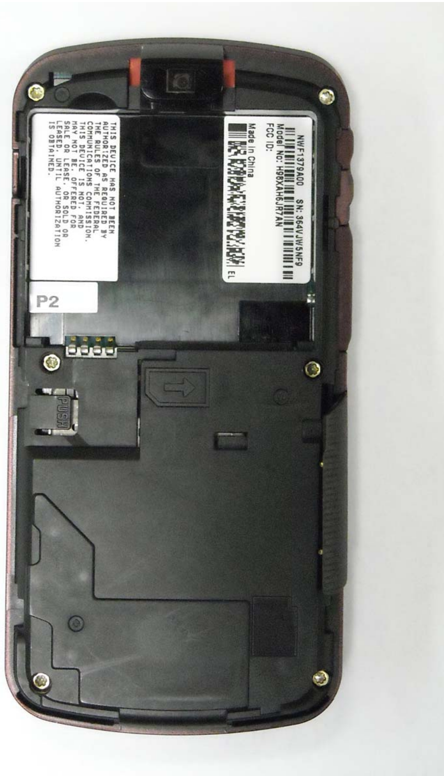
Figure 3-8. Interior Compartment of radio – Battery Removed
