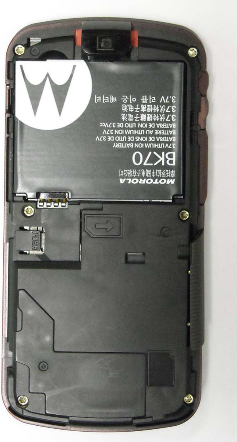
Figure 3-7. Interior Compartment of radio – Battery in Place
