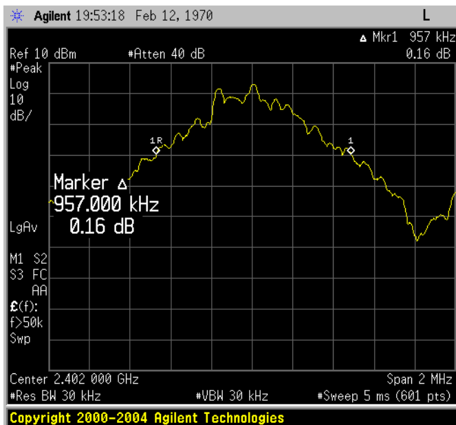
Figure 6c.2-1: Plot of 20 – dB bandwidth
