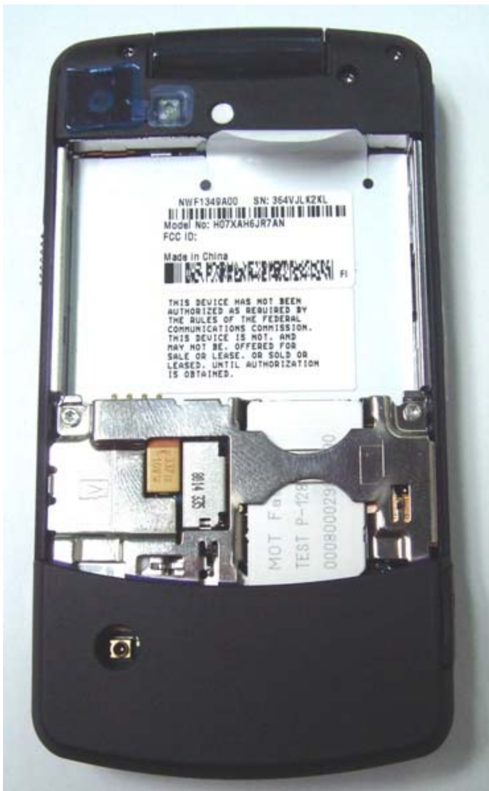
Figure 3-6: i9 Rear View (Battery Removed)
