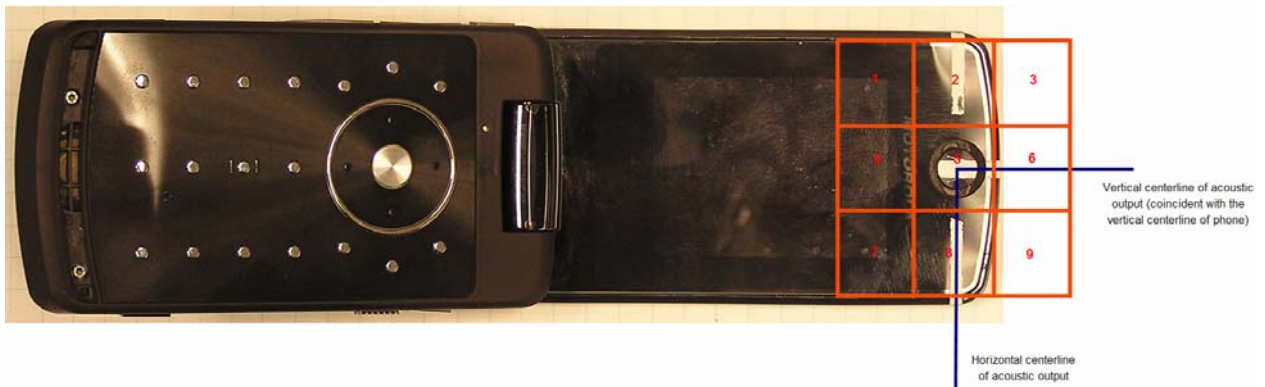
Figure 2. Phone Front - Orientation and Measurement Plane for RF Emissions Testing
