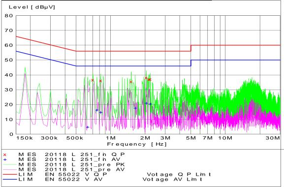
GSM 850 Channel 251 - Tx Mode - Line Coupling
