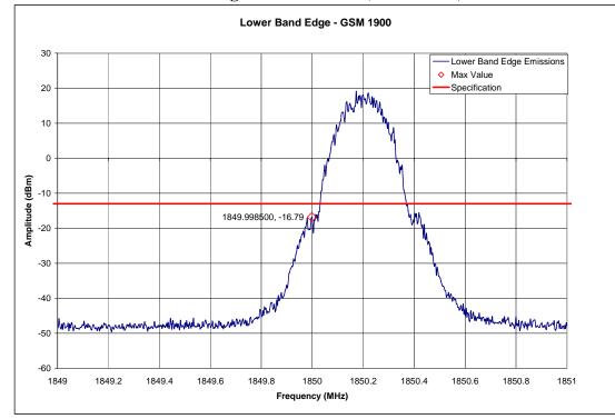
GSM 1900 – Lower Band Edge – Channel 512 (1850.2MHz)
