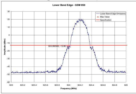
GSM 850 – Lower Band Edge – Channel 128 (824.2MHz)
