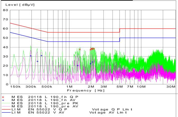
GSM 850 Channel 190 - Tx Mode - Line Coupling
