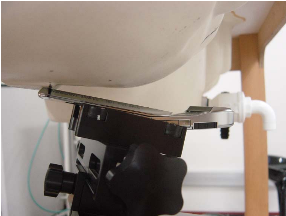
Figure7: Phone Against the Head Phantom (15° Tilt - Phone Open)
