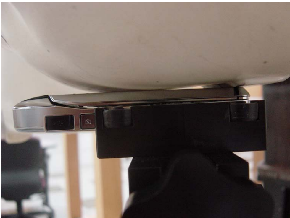
Figure4: Phone Against the Head Phantom (Cheek Touch - Phone Close)
