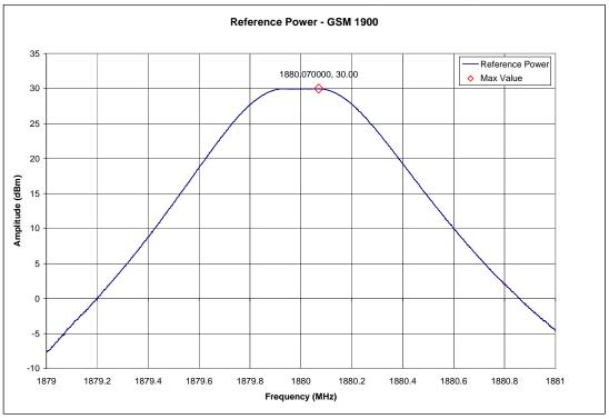
GSM 1900 - Occupied Bandwidth - Channel 661 (1880.00MHz)
