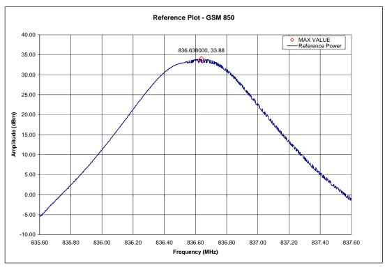
GSM 850 – Occupied Bandwidth – Channel 190 (836.6MHz)
