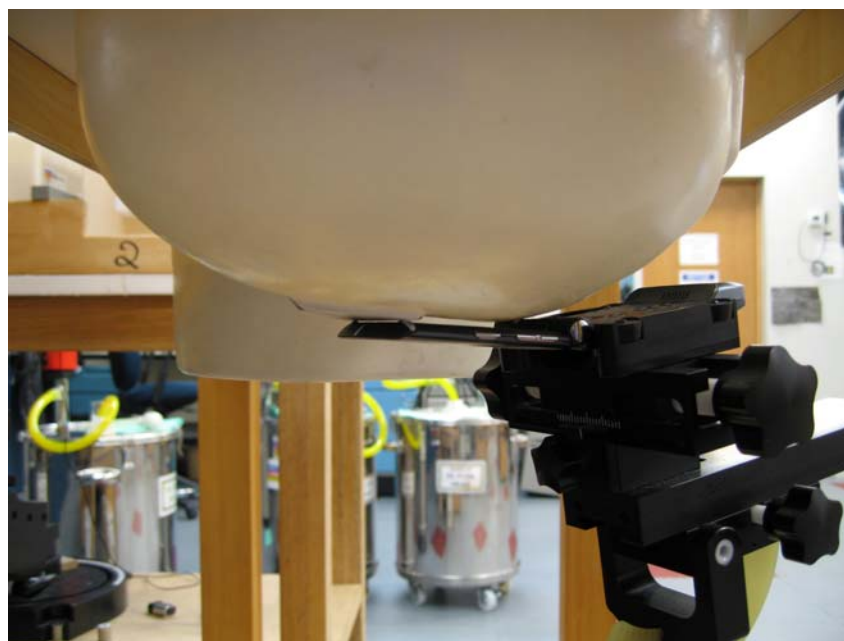
Figure 6 – Transceiver against head, Cheek Touch position
