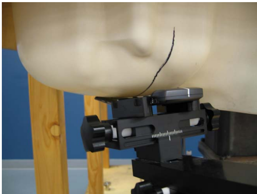
Figure 5 – Transceiver against head, Cheek Touch position
