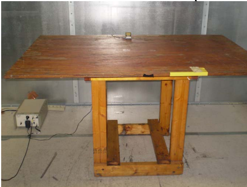
AC Line Conducted Emissions Measurement Setup.
