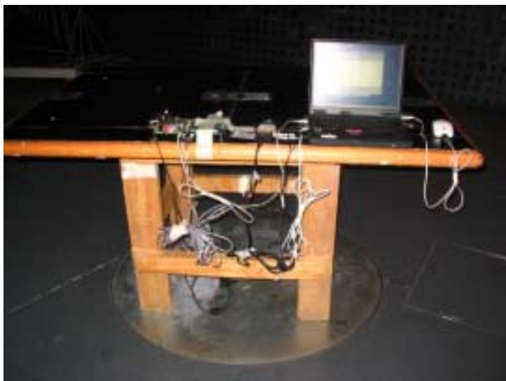
Photograph 7.2.2 Setup for radiated emission measurements, EUT cabling
