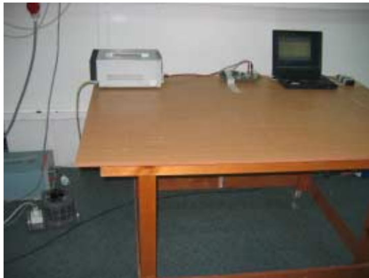
Photograph 7.1.1 Setup for conducted emission measurements
