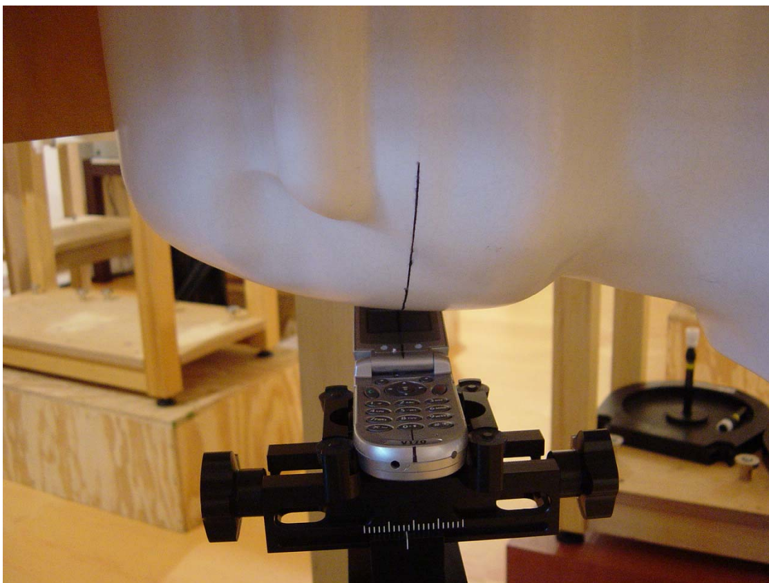
Figure 7: Phone Against the Head Phantom (Front View – Tilt)
