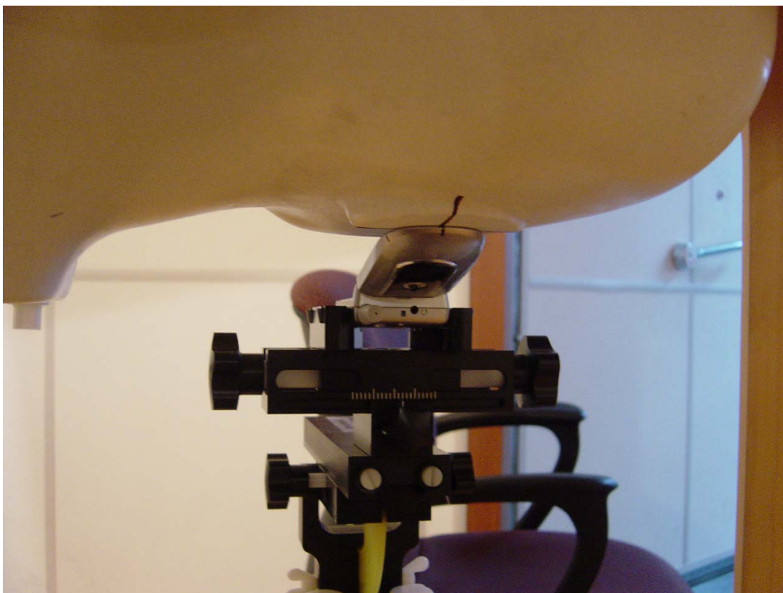
Figure 8: Phone Against the Head Phantom (Back View – Tilt)
