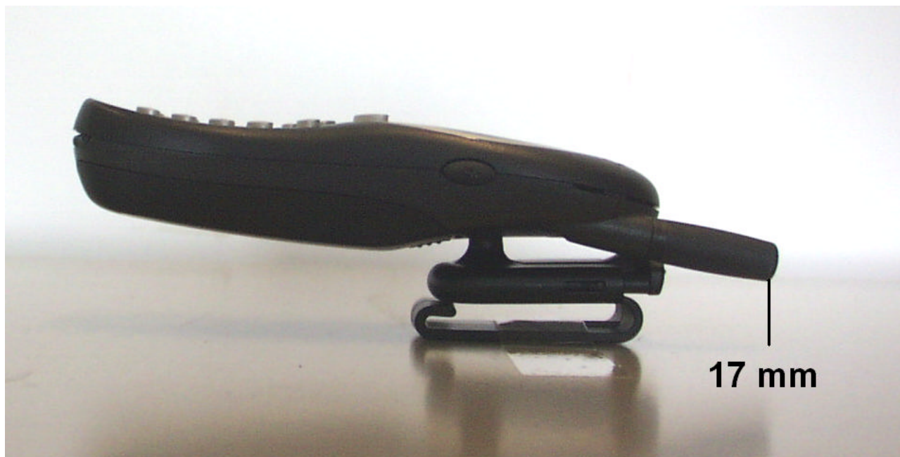
Figure 17. Distance of the Antenna (Extended) to the Base of the Flat Phantom
