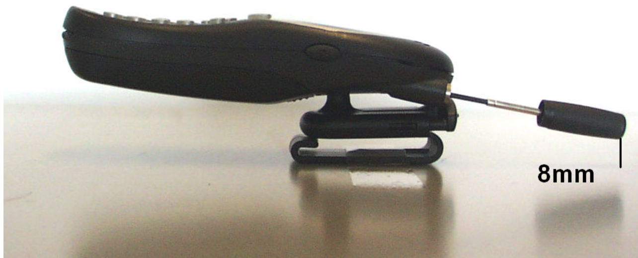
Figure 17. Distance of the Antenna (Extended) to the Base of the Flat Phantom
