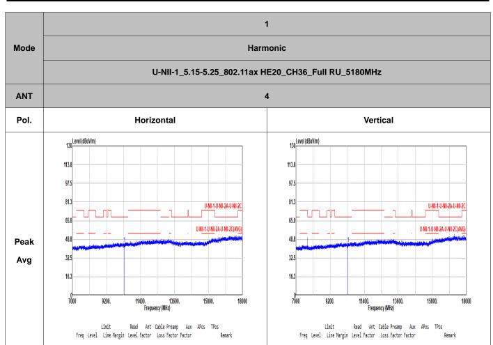
Note: For all plots above, the over limit line signals are Fundamental signal which can be ignored
