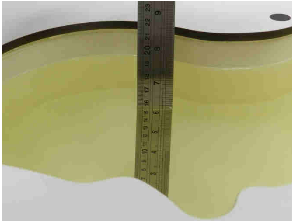
Fig 11.1 Photo of Liquid Height for Head SAR
