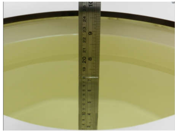
Fig 11.2 Photo of Liquid Height for Body SAR
