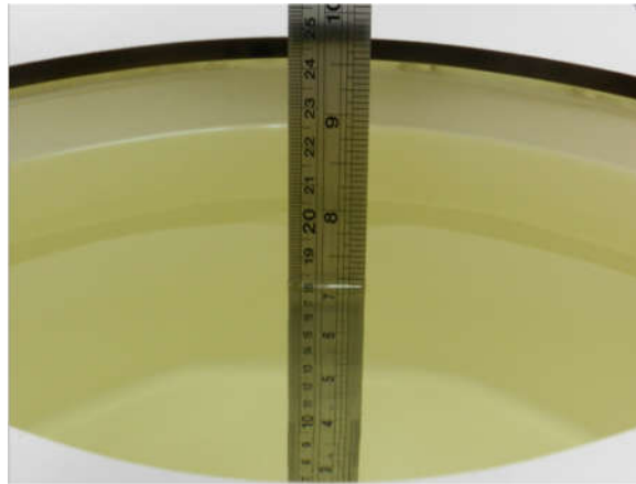
Fig 11.1 Photo of Liquid Height for Body SAR
