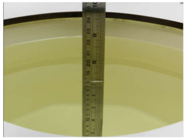
Fig 11.2 Photo of Liquid Height for Body SAR
