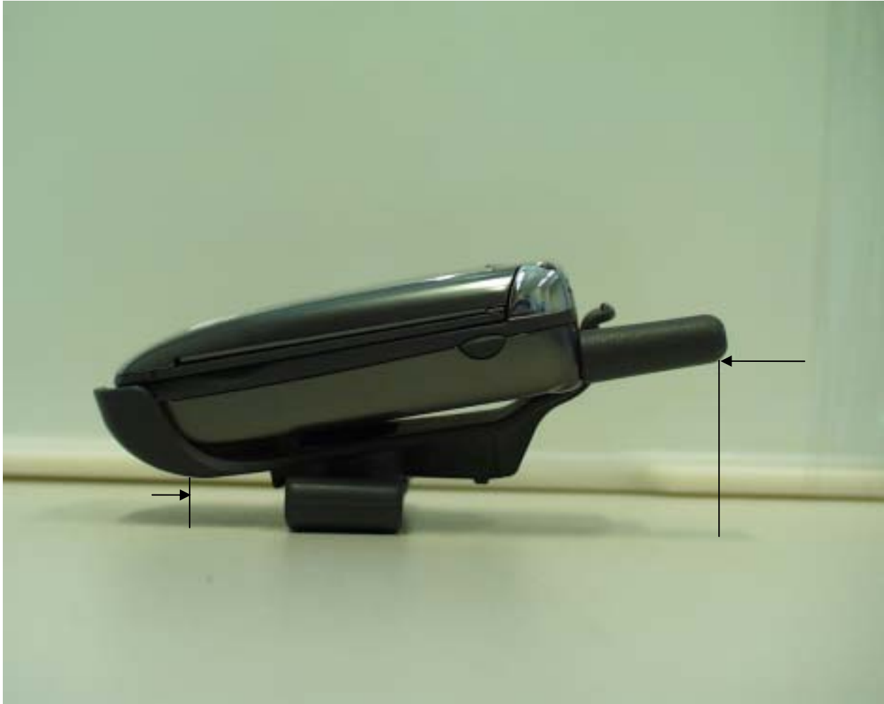
Figure 11 . Separation Distance of 25 mm from Tip of Antenna to Flat Phantom and 8 mm from the bottom of the clip when rotated +90° (Clockwise Direction)
