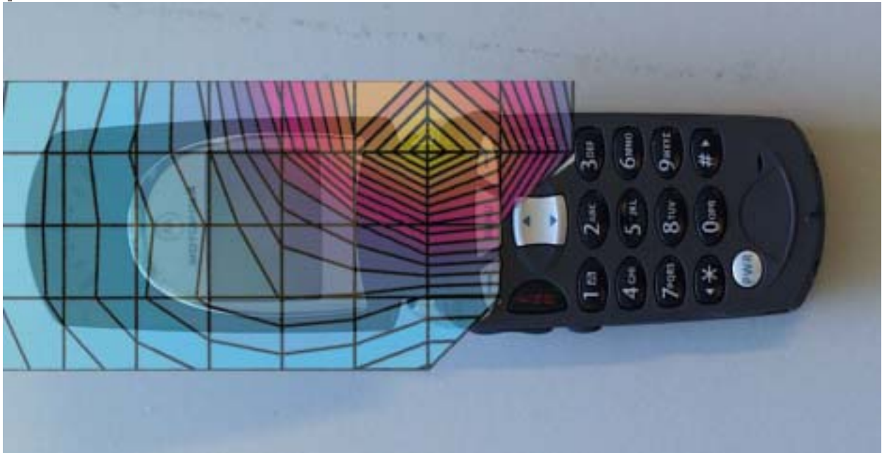
Figure 1. Typical 800MHz Head Adjacent Contour Overlaid on Phone (Cheek Touch)
