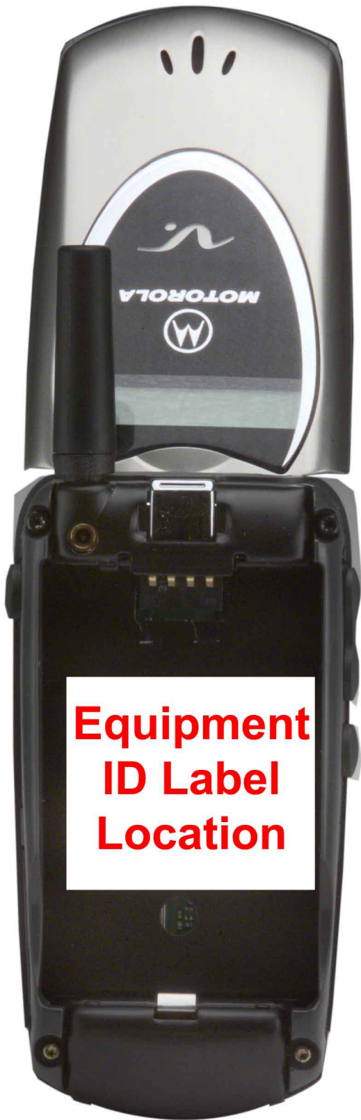
Rear View, Flip Opened with Battery Removed to Show Equipment ID Label
