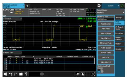
3DH5 on time (Count Pulses) Plot on Channel 00
