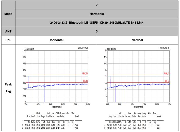
Note: the highest signal over limit is co-location fundamental signal.
