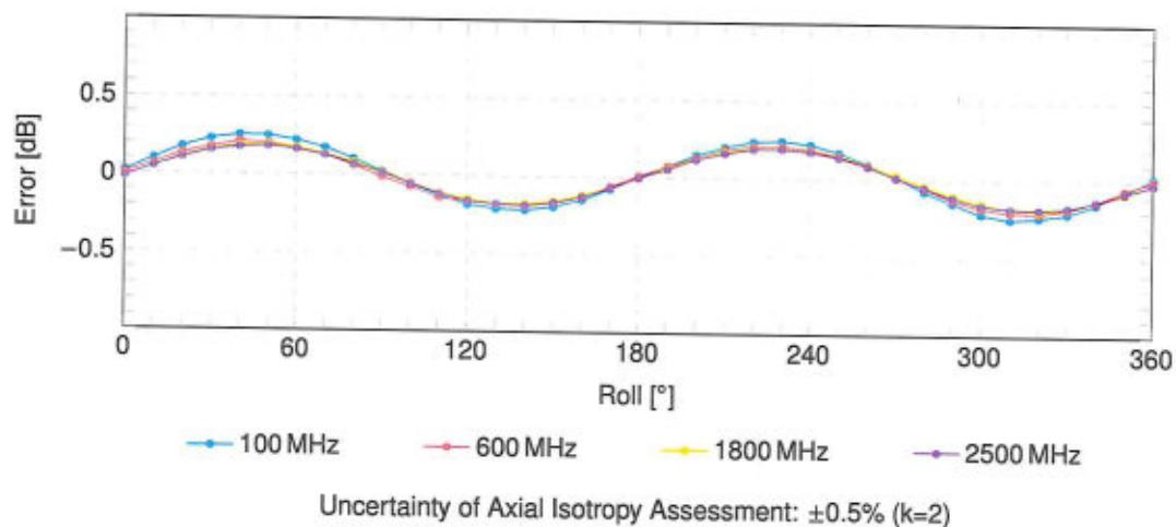
**Receiving Pattern ( $\phi$ ),  $\vartheta = 90^\circ$**
