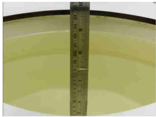
Fig 11.2 Photo of Liquid Height for Body SAR
