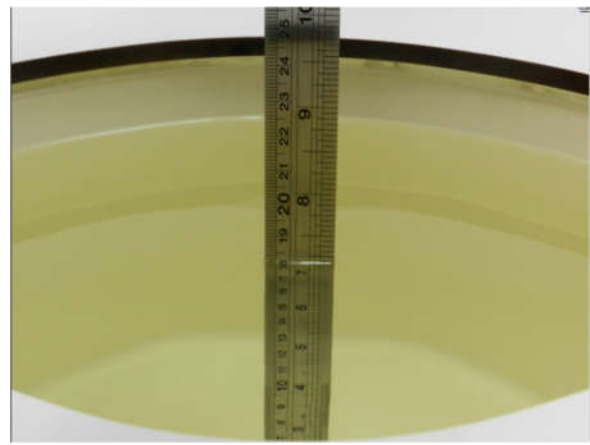
Fig 11.2 Photo of Liquid Height for Body SAR
