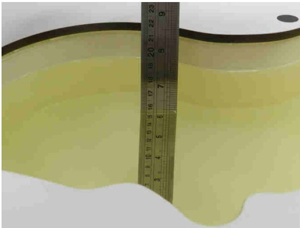
Fig 11.1 Photo of Liquid Height for Head SAR
