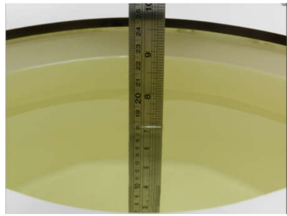
Fig 11.2 Photo of Liquid Height for Body SAR
