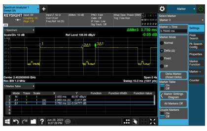
3DH5 on time (Count Pulses) Plot on Channel 39
