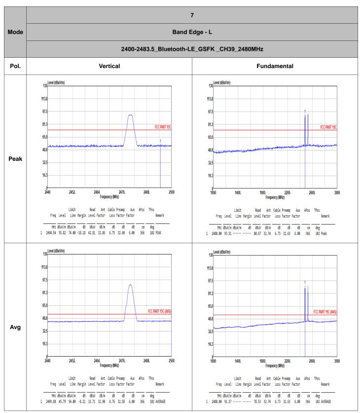
Note: the highest signals over limit are BLE + WWAN co-location fundamental signals.
