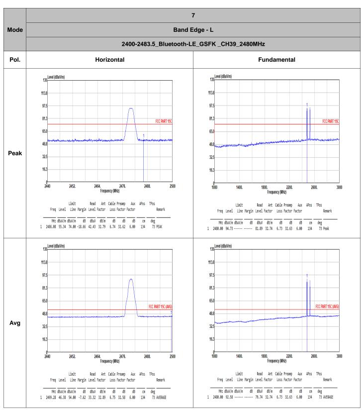
Note: the highest signals over limit are BLE + WWAN co-location fundamental signals.
