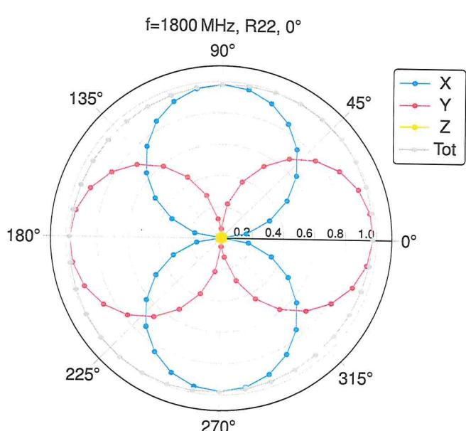
**Receiving Pattern ( $\phi$ ),  $\vartheta = 90^\circ$**
