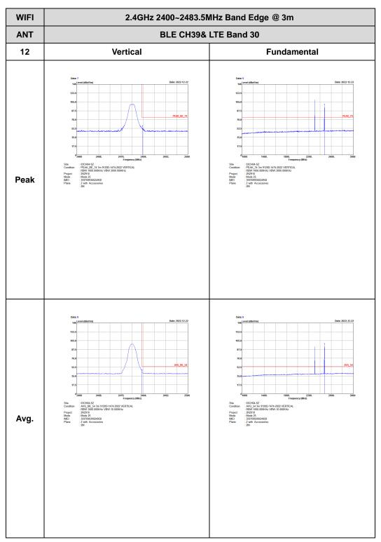
Remark: The two highest signals are BLE and LTE B30 fundamental signal in the Fundamental plot.
