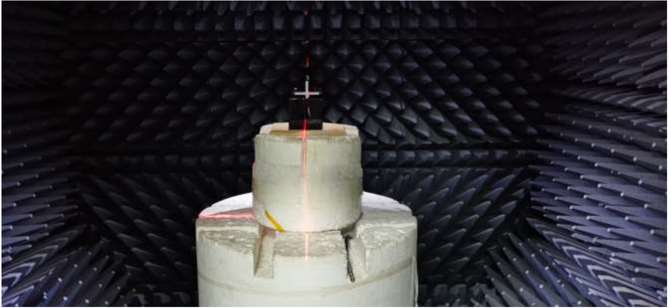
Antenna Gain test erection photo
