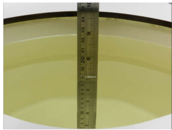
Fig 11.2 Photo of Liquid Height for Body SAR
