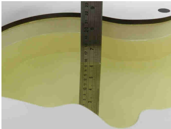
Fig 11.1 Photo of Liquid Height for Head SAR
