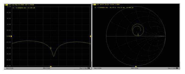
Dipole Verification Data> D3900V2, serial no. 1048
