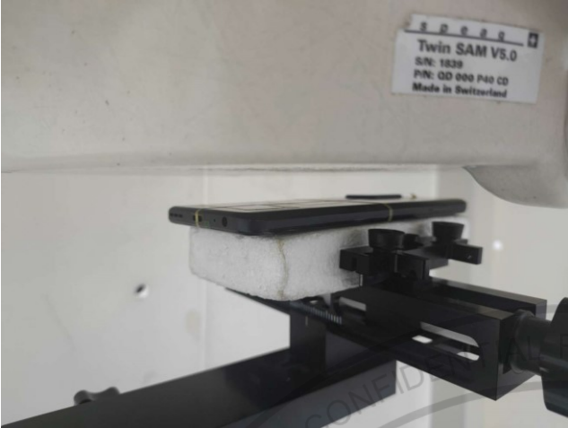
Back, Test Separation 23 mm
