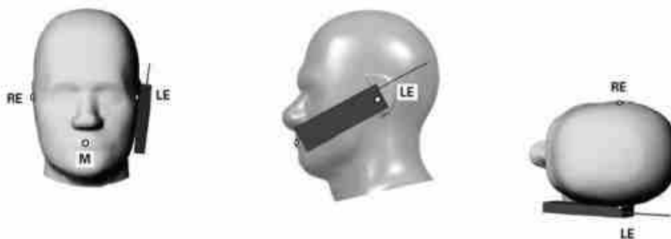
Fig 12.2.3 cheek or touch position. The reference points for the right ear (RE), left ear (LE), and mouth (M), which establish the Reference Plane for handset positioning, are indicated.
