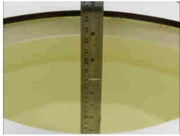
Fig 11.2 Photo of Liquid Height for Body SAR
