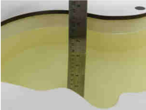
Fig 11.1 Photo of Liquid Height for Head SAR
