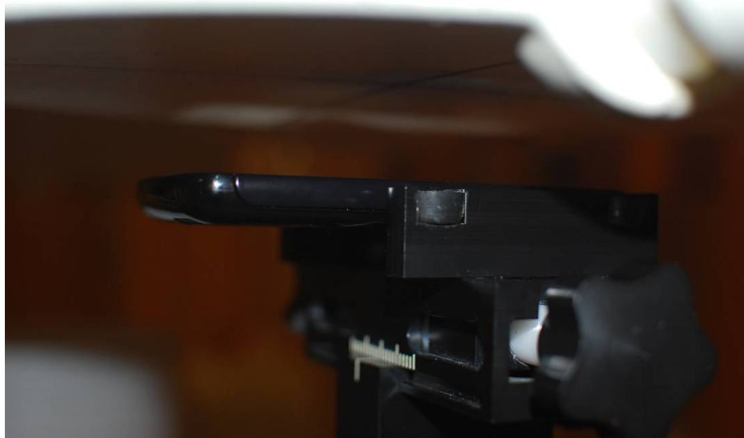
Figure 18-4 SAR Test Setup Front 2.5 cm
