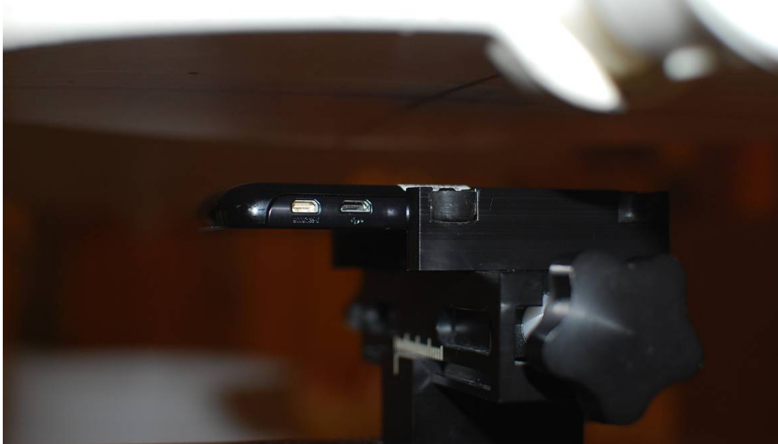
Figure 18-2 SAR Test Setup Back 2.5 cm
