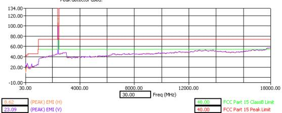
30 MHz – 18 GHz Low Channel Dual Polarization Y
