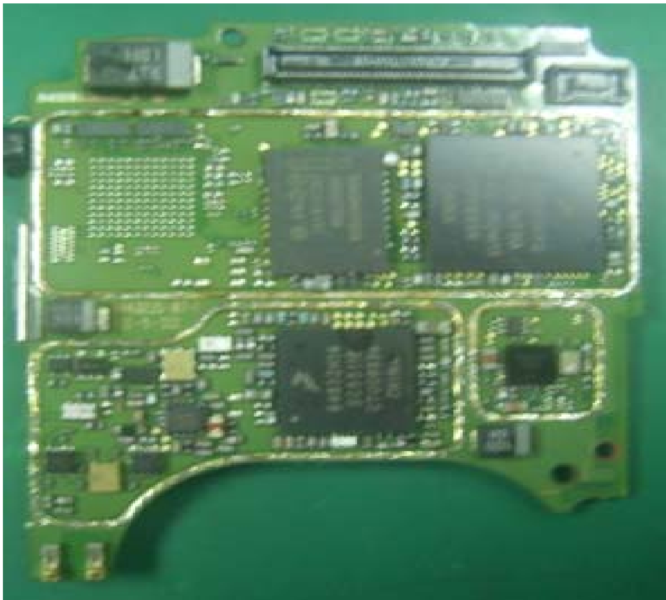
Photograph 9-2: Front side view of radio product Keypad PC Board (Shields Removed).
