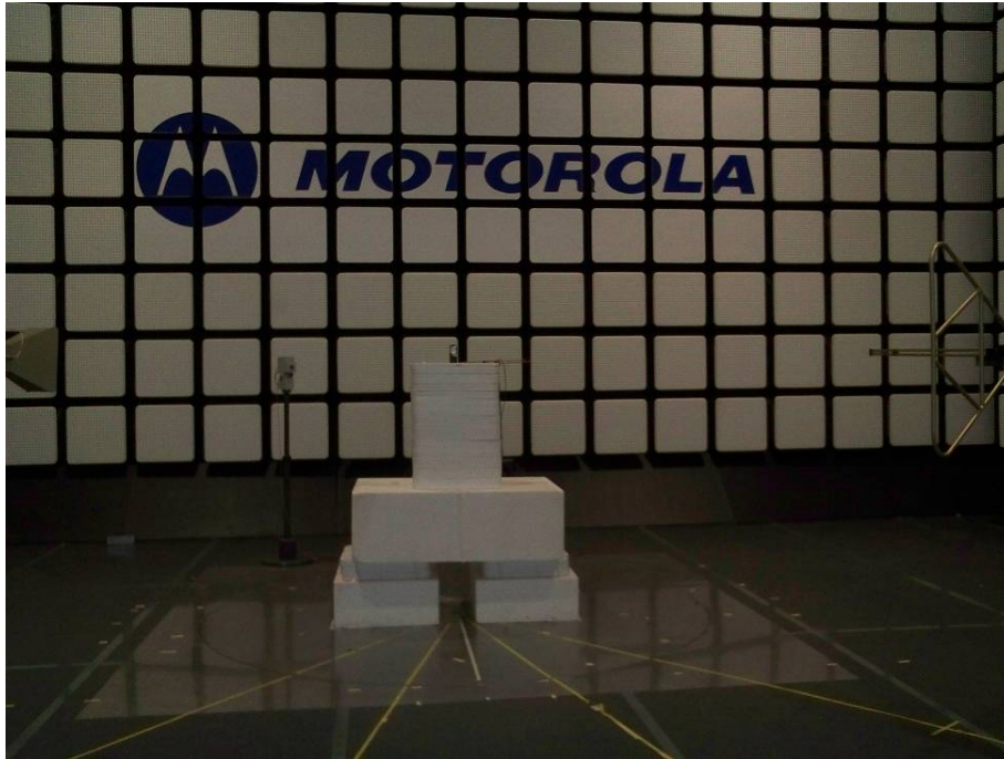
22725-1, IHDP56JQ1 setup in semi-anechoic chamber – front view (30 MHz-18 GHz)
