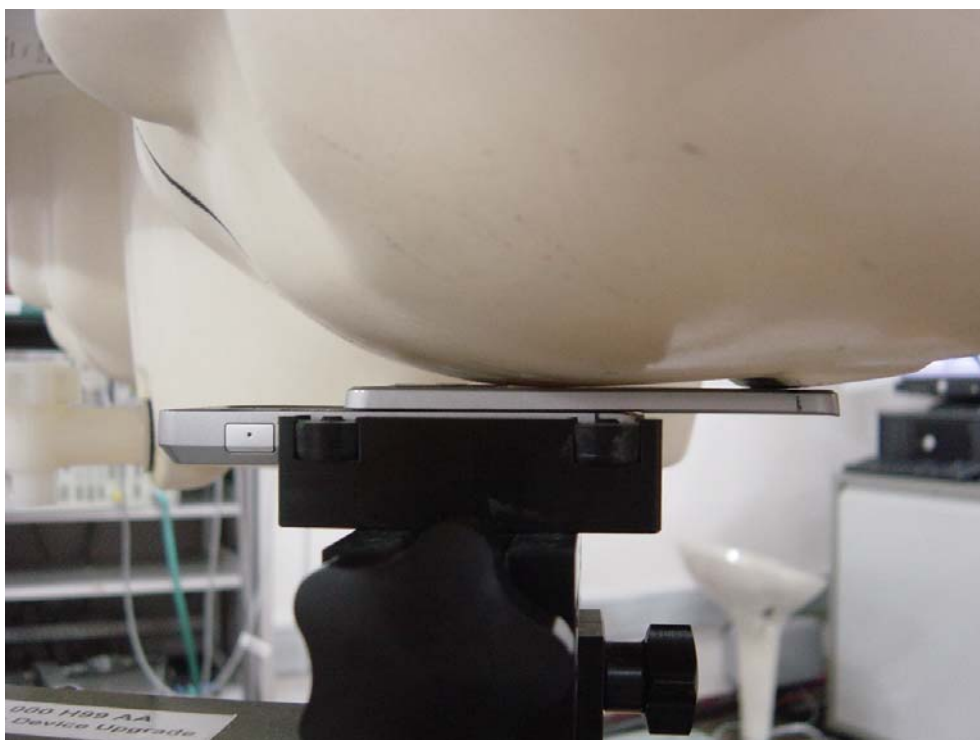
Figure 6: Phone Against the Head Phantom (Cheek Touch - Slider Open)
