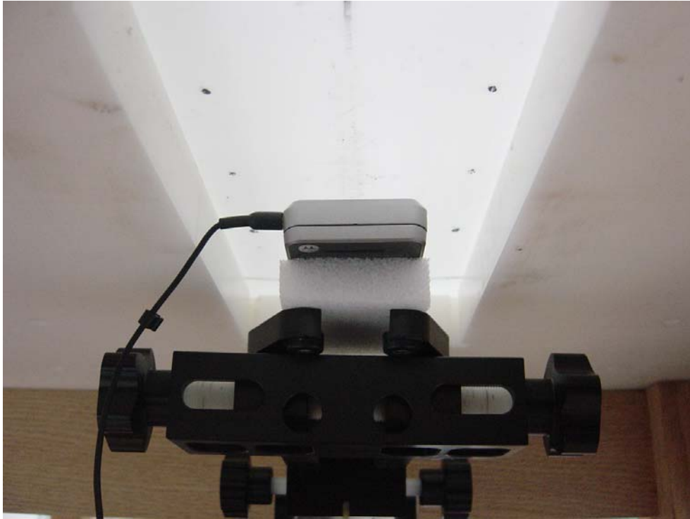
Figure 9: Phone Against the Flat Phantom
