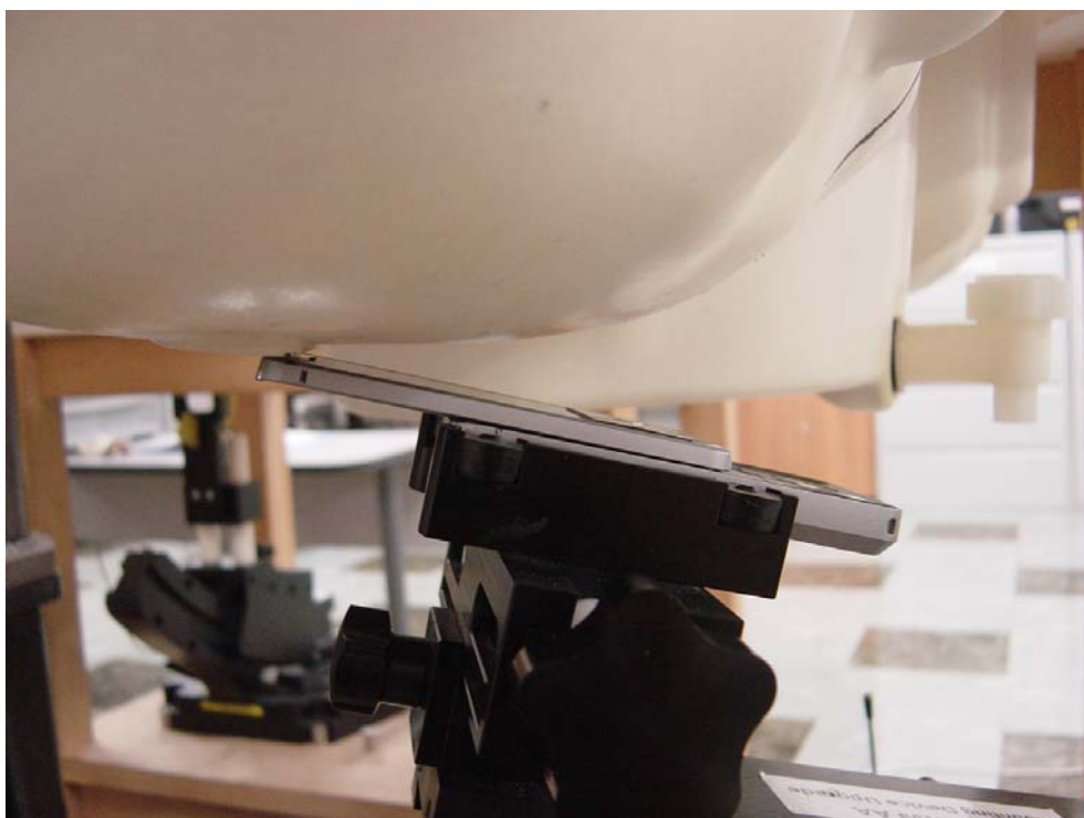
Figure 8: Phone Against the Head Phantom (15° Tilt - Slider Open)
