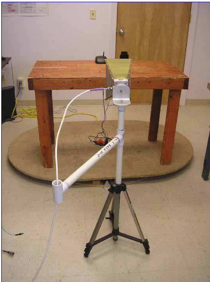
Photograph 2. Intentional and Spurious Emission Limits Test Setup
